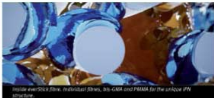
A cross-sectional view of everStick fibre. Silanated glass fibres are impregnated with PMMA and bis-GMA.
